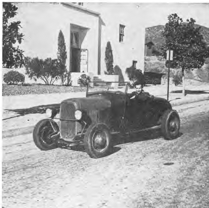
Gertie Schirmeister tears around in his A V-8 roadster. The motor is ported and relieved with milled heads and semi-cam.
