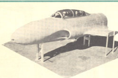
4. Production planning begins with a mock-up or full scale model of the plane. Here manufacturing methods are planned and location of parts is tested for ease of manufacture, comfort, access.
