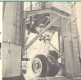
5. Torture tests of parts to go into the completed plane must prove they have many times the strength required of them in service.
