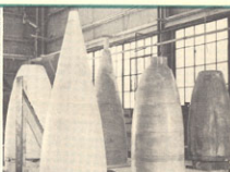
7. Meanwhile, tool designers build plaster molds for dies and patterns, jig and fixture builders go to work, and engineers finish plans for the many parts.
