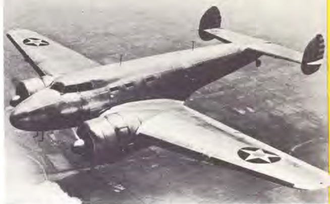
XC-35 Electra was first pressurized plane. It won 1937 Collier Trophy for stratosphere hops.
