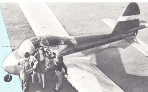
Two-place Big Dipper had clean design, propeller behind tail.
