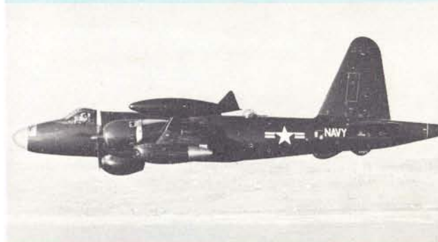
With enlarged cockpit, "stinger" tail, new P2V-7 illustrates design progress.
