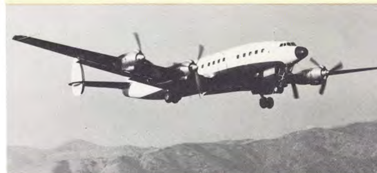
Mighty 1649A Starliner shown above on first flight has 150 foot wing, 6000 mile range. Below, crowds welcomed Eisenhower when he arrived at Lockheed Air Terminal in presidential Connie, the Columbine III.
