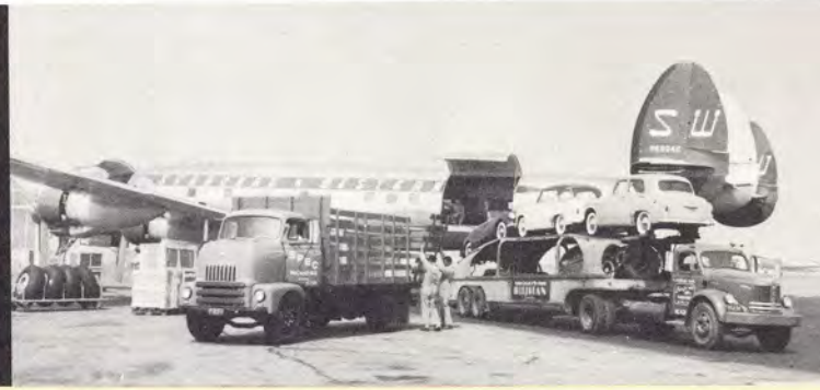
Quickly convertible for either passenger or cargo service, Model 1049H had first flight in late 1956. It has 150,000 pound gross weight, 17-20 ton payload.
