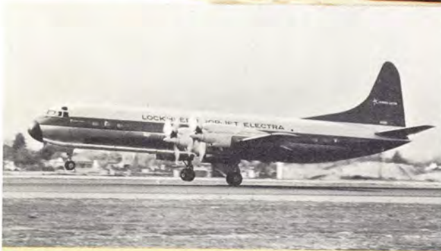
Fitted with four Allison Model 501 prop-jets, Electra lifted wheels during taxi test. Plane will carry 66 to 91 passengers, fly 400 mph.
