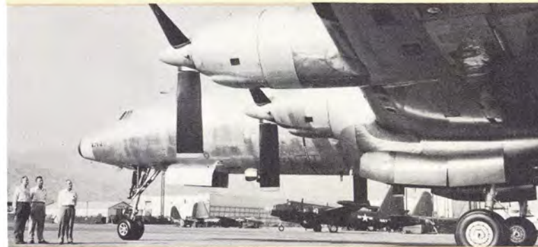
Broad propellers and sleek nacelles are features of Navy's R7V-2 (above), Air Force's YC-121F Connies, prop-jet powered and capable of better than 400 mph.
