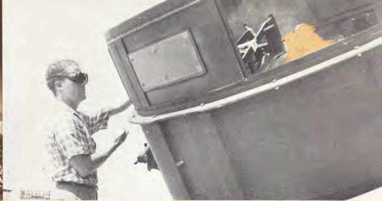
Solar furnace is among test equipment developed by Missile Division to accelerate progress of Navy's top priority weapon, the solid-propellant Polaris.
